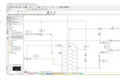
Thanks to integrated design checks, individual P&ID drawings or the entire project can be checked for completeness, plausibility and accuracy. Customized design checks can be added quickly and easily.
