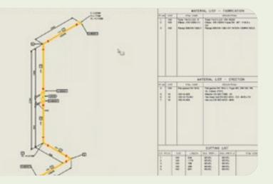
The pipeline illustrations as well as all relevant information – such as dimensions, forged hatching, annotations – are created automatically via preset parameters (styles), which can be configured individually.
